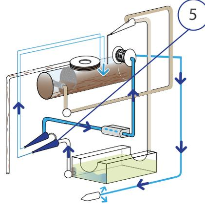
**FINISHING CYCLONES** provides further refinement, capturing and discharging any residual impurities. After going through the GENESIS 5 stages of separation, the recycled water is free of all materials larger than 50 microns. The small size, quantity and consistency of anything remaining is not able to damage your plumbing, hoses or nozzles.
