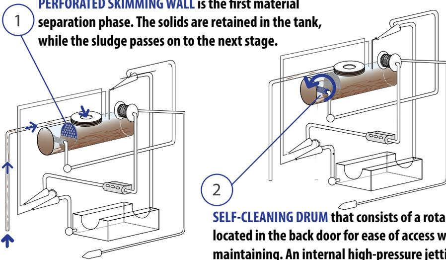
**PERFORATED SKIMMING WALL** is the first material separation phase. The solids are retained in the tank, while the sludge passes on to the next stage.
