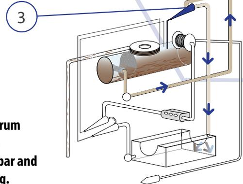
**EXCLUSIVE 5 COMPARTMENT SETTLING TANK** separates fats, oils, and grease (FOG) as well as solids, separating the water from the impurities it contains. This sedimentation tank is the stage that guarantees the high quality water produced by the GENESIS recycling system.
