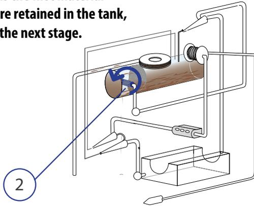
**SELF-CLEANING DRUM** that consists of a rotary drum located in the back door for ease of access when maintaining. An internal high-pressure jetting bar and brass scraper keep the drum clean while working.
