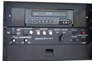
**Sewer Inspection System** includes: rack mounted controls and a video recording device (VHS, digital, or computer with software) in a shock resistant/weather tight enclosure, a camera head (self-leveling or 360 degree view), and a viewing monitor (with optional on-screen footage display and audio recording device) all stored in the heated rear compartment.
