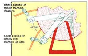
**Automatic Level Wind** with Up/Down Action and a Pendant Control allows for safe, clean, and hands-free hose operation away from traffic.
