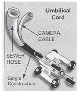
**Umbilical Cord\*** is a single unit construction of 5/8" sewer hose and multi-conductor camera cable wrapped in a protective, repairable molded casing. The 500' Umbilical Cord allows for easy jet tv operation working just like a sewer cleaning nozzle.
